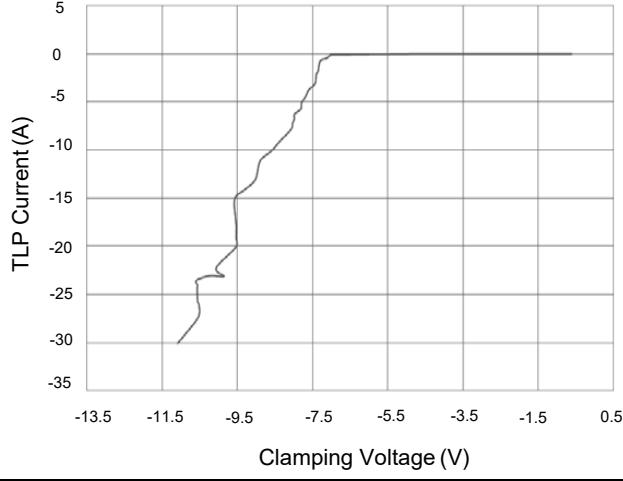
**Figure 5: ESD Clamping(IEC61000-4-2:+8kV)**
