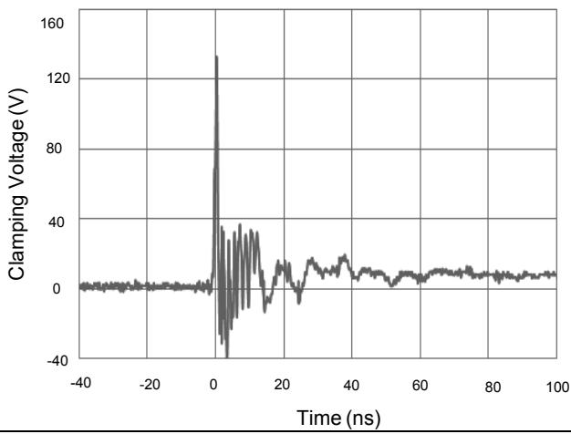
**Figure 6: ESD Clamping(IEC61000-4-2:-8kV)**
